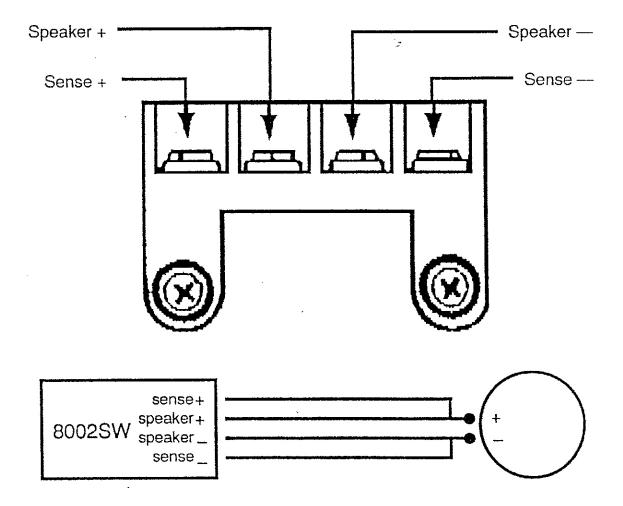
**NOTE:** IN ADDITION TO THE IMPEDANCE REQUIREMENTS THAT MUST BE MET FOR SPEAKERS USED WITH THIS AMPLIFIER, THE COMBINED CONTINUOUS POWER HANDLING CAPABILITY OF THE SPEAKER (S) USED IS RECOMMENDED TO BE AT LEAST **1000 WATTS** FOR SAFE OPERATION.
